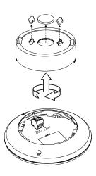
2. Thread the DALI cable through the housing mounting, and screw the Remove the DALI connector block from the receiver housing.
