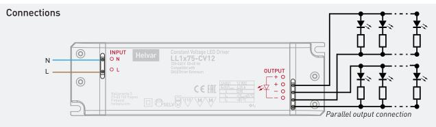
Attention: If using LL1-CV-DA or LL1-CV-SC control units to control LED load with this driver, make sure the total output current from the LL1x75-CV12 driver does not exceed 5 A (60 W)!
