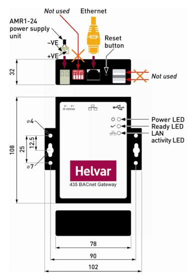
Note: Typically, individual systems (energy control, lighting, boiler and air-conditioning systems, etc.) are measured separately for CO<sub>2</sub> accountability. Therefore, installing the BACnet Gateway and combining the various systems can help an effective BeMS be more energy efficient and comply with national building regulations.
